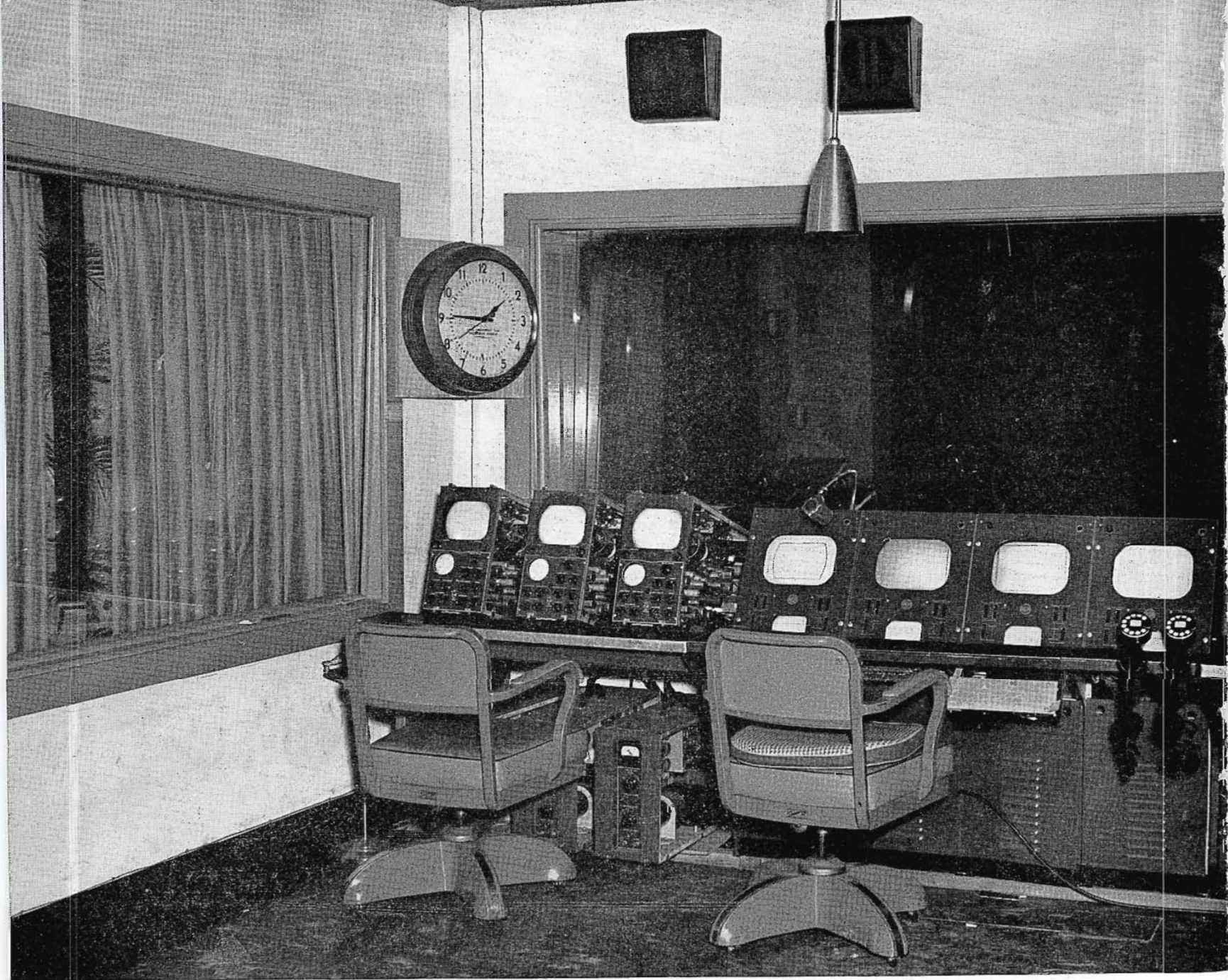
FIG. 7. One side of the studio control room contains (at left) three camera controls for the three field-type cameras used in the studio. Other equipment visible, left to right, includes line monitor and TS-10A Camera Switching System, preview monitor, and two film camera controls. Audio console and equipment racks are not shown. Side window joins clients' viewing room.
