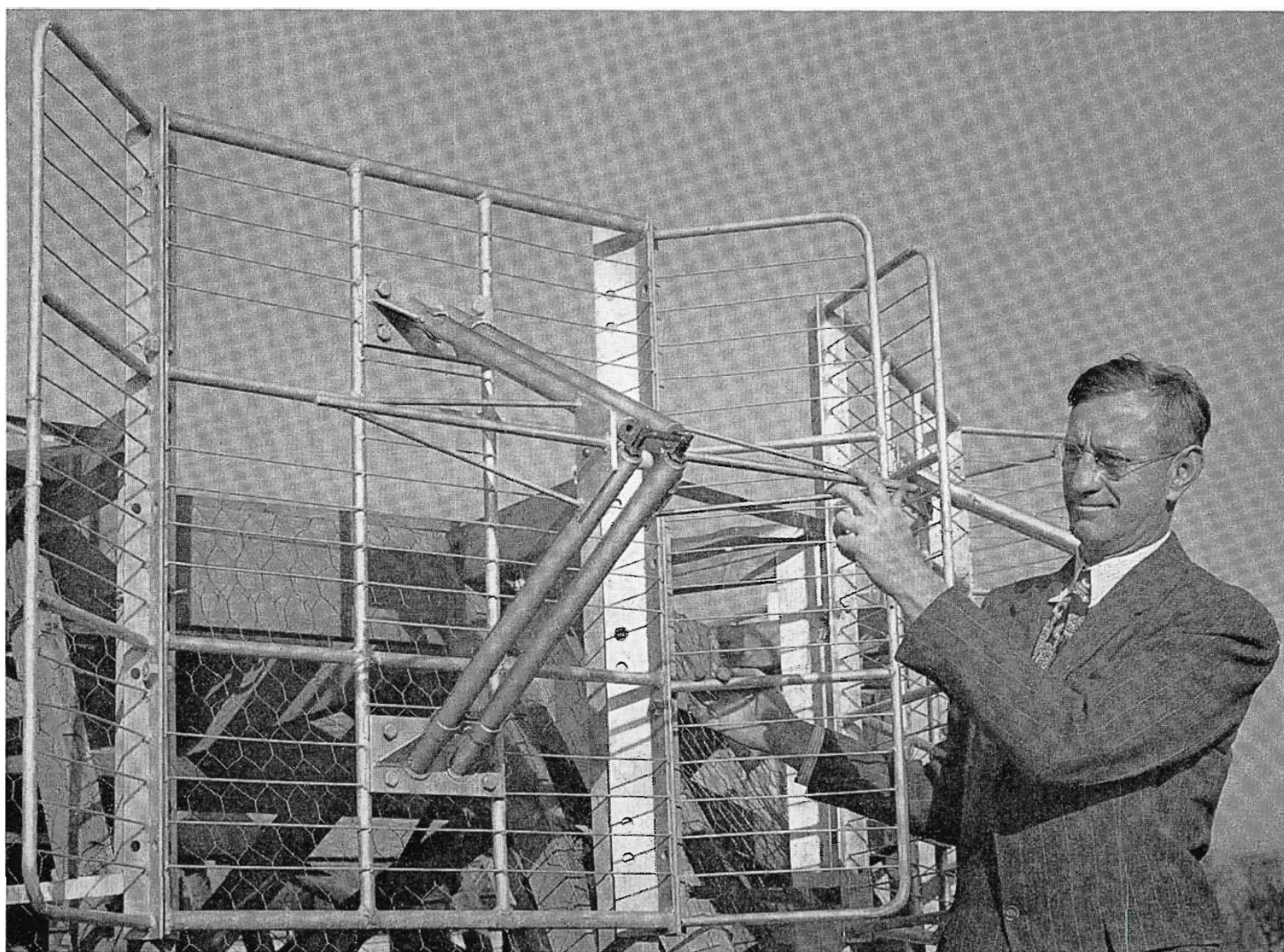
FIG. 1. L. J. Wolf examines developmental model of RCA's new Supergain Antenna. Reflecting screens on sides are used to reinforce forward radiation. Wire screen behind antenna used during tests simulates sustained tower or building.
