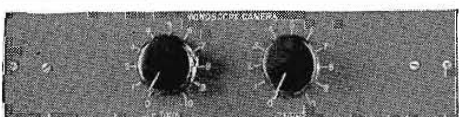
Monoscope Camera Control, MI-26248. Provides remote control of video gain, and focus of monoscope camera. Includes 2 potentiometers wired to terminal board.
