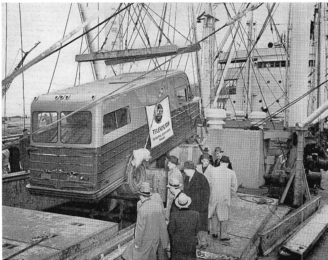
(RIGHT) Lowering the mobile unit into the hold of MORMACYORK at Philadelphia Port. Equipment, which was shipped several months ago, is now being installed and is expected to be in operation by mid-summer. Station will operate on U. S. Channel 3 (60-66 mc) and use U. S. standards of 525 lines and 60 fields.
