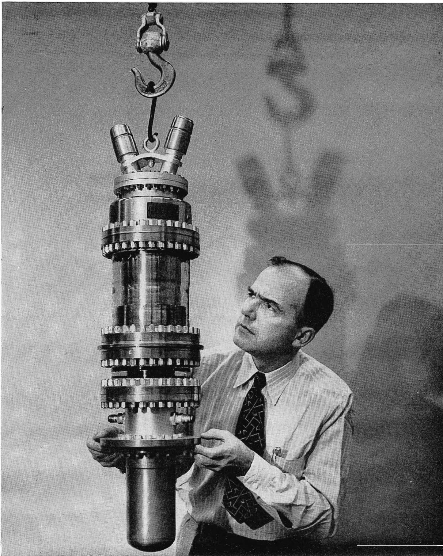
FIG. 1. RCA's new "Super-Power Beam Triode," which is capable of 500 kilowatts output and which has been tested at 1,000,000 watts input, is shown above with Dr. L. P. Garner, head of the Advance Development Lab of the RCA Lancaster, Pa. tube plant, in which the tube was developed. Despite its enormous power output, the new tube is of relatively compact design, weighing only 135 pounds and measuring only 38\frac{3}{4} inches in length. Present applications of the new tube are in high power CW applications and International Broadcast Service.
