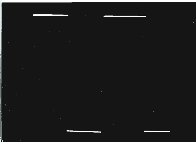
FIG. 35. Signal across R_o with 6SN7 plate coupled output. R_o = 100 \text{ ohms} R_L = 10,000 \text{ ohms} C = 125 \text{ MFD}
