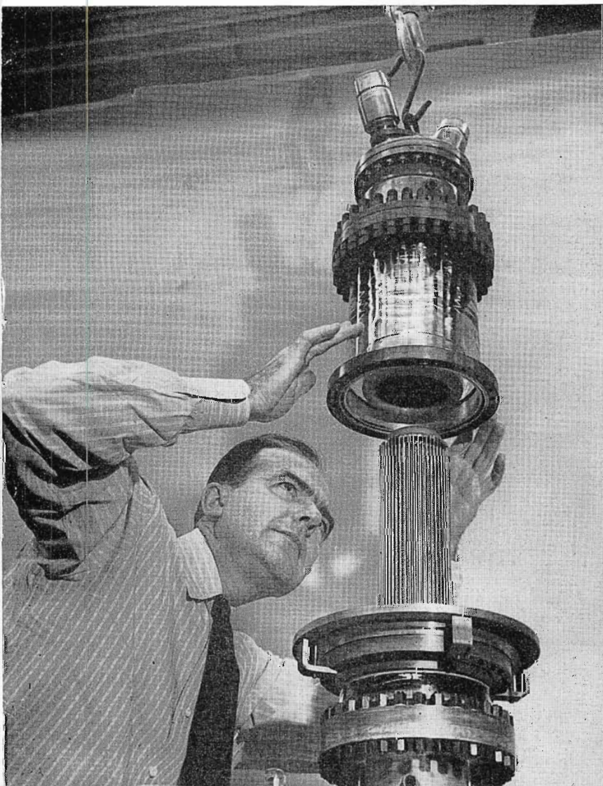
FIG. 2. The unique internal structure of RCA's new "Super-Power Beam Triode" 5831 is shown below, as Dr. L. P. Garner, head of the RCA Lancaster tube plant's Advance Development section, directs the lowering of the anode-envelope assembly into position. The high power capability of the new tube is due largely to the arrangement of 48 separate triodes in relatively small space.
